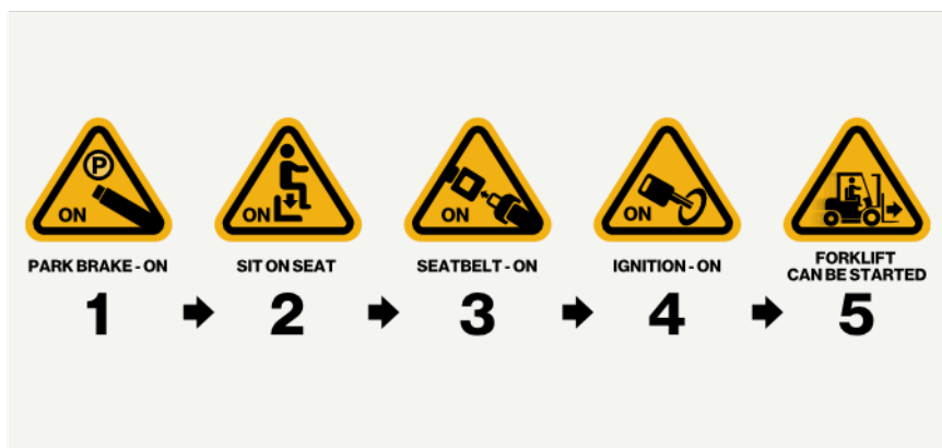
Figure 11: An example of a label on a forklift to show the procedure for using a sequential interlocking seatbelt.
